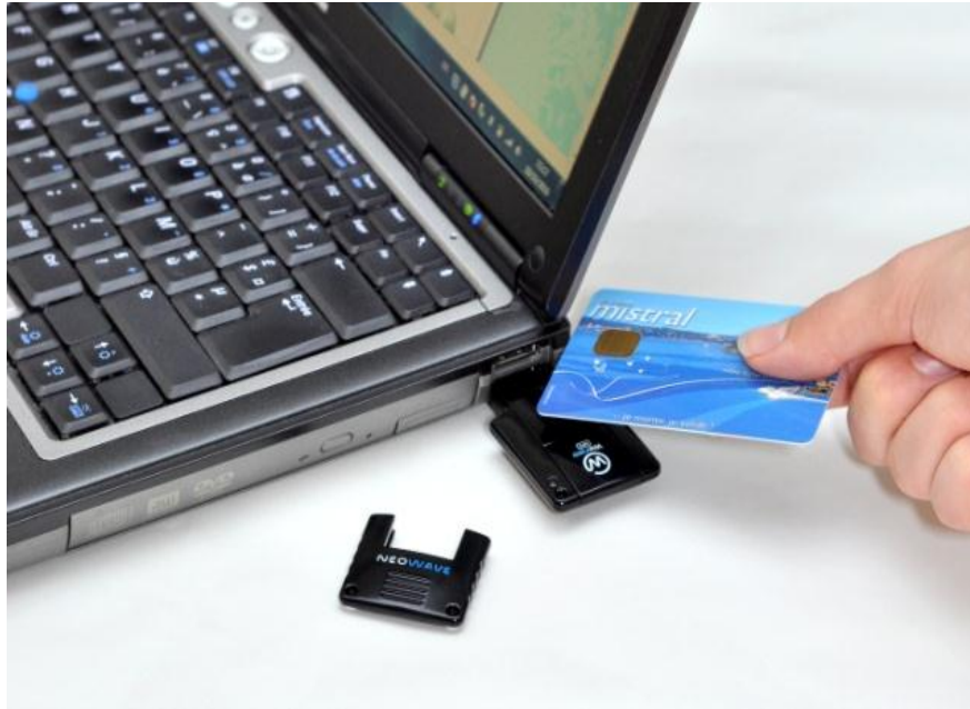
Weneo NFC: NFC contactless reader
